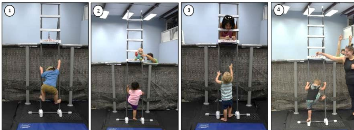
Figure 3. Child Subjects Unable to Climb Pool Ladder with Removable Steps (Test Trial 1)
