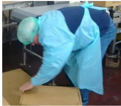
Figure 1: Existing handling posture required when moving the bottom row of boxes
