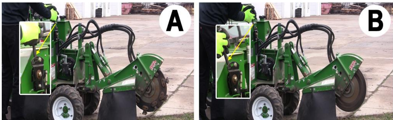
Figure 3. Cutter Wheel Control Lever Testing (Cutter Wheel Disengaged in A and Engaged in B)
