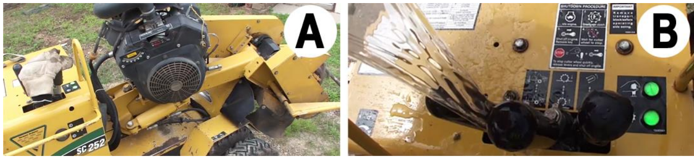
Figure 5. Capacitivity-Sensing OPC Testing (Wet Glove Detection Error in A and Water Detection Error in B)
