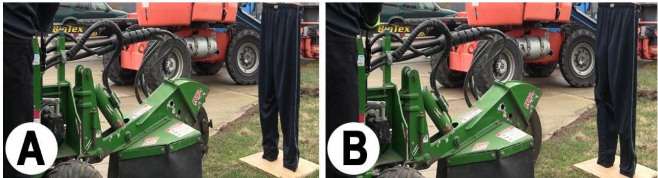
Figure 2. Pants Test Fixture (Cutter Wheel Disengaged in A and Engaged in B)
