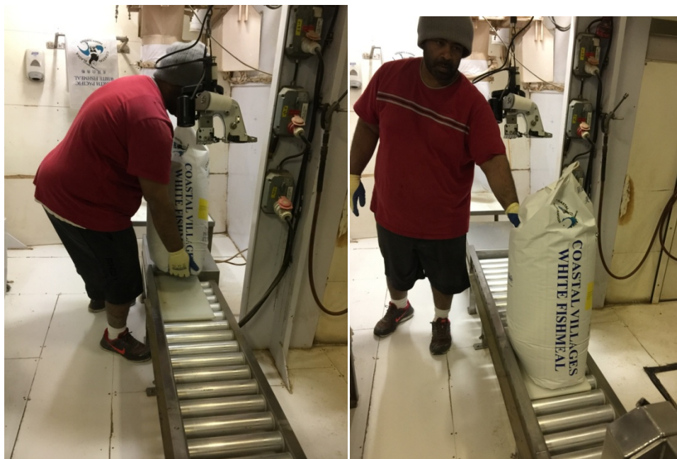
Figure 13. Rigid plastic used under each bag to ease sliding.
