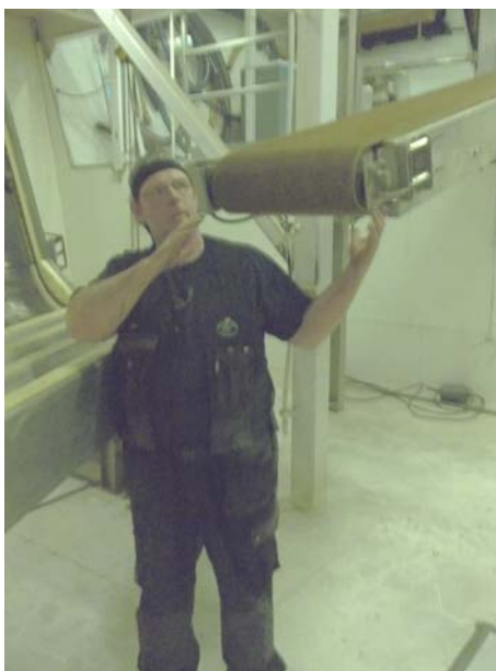
Figure 5. Powered conveyor in lower storage area has some height adjustability for different employee statures. Shown here at 69" H for comfortable shoulder loading for this employee.
