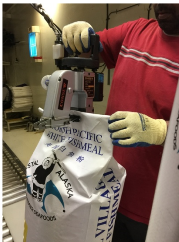
Figure 9. Sewer machine too high and too far to the left (from employee perspective), causing high risk shoulder posture.
