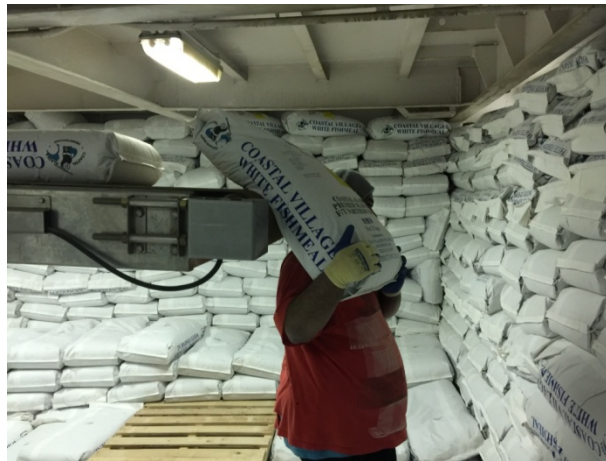
Figure 14. Powered conveyor in upper storage area set at height that avoid a squat lift and allows bag to easily be positioned on employee's shoulder.
