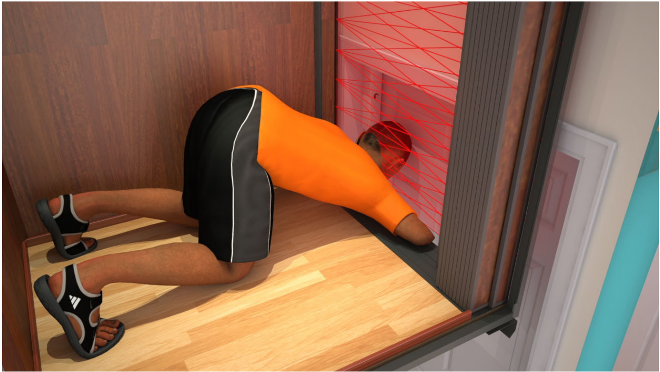
Figure 4. Elevator Light Curtain Accident Prevention.
