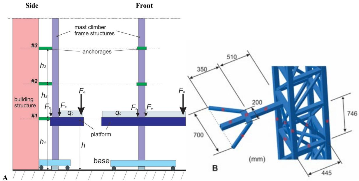
**Figure 1.** Conceptual design of the numerical simulations. (A) The simulation model consists of three parts: a base, a mast, and a platform. The mast has a height of 33.60 m and is connected to the construction building via three anchorages. The anchorage locations:  $h_1 = 12.7$  m and  $h_2 = 9.05$  m. (B) Detailed anchorage structure.
