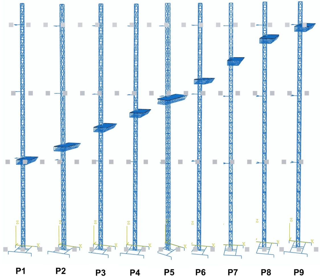
**Figure 2.** Finite element models of the mast climbers when the work platform operates at different heights. P1, P2, ..., P9 represent nine operation positions (heights).
