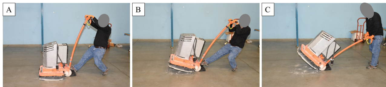
Figure 1. Concrete grinding machine tilting process.
