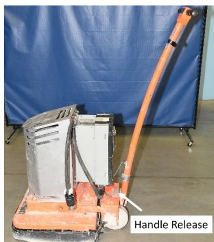
Figure 4. Location of concrete grinder's handle release mechanism.
