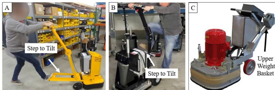
Figure 5. Alternative machine designs employing step to tilt (A & B), and removable counterweights (C).
