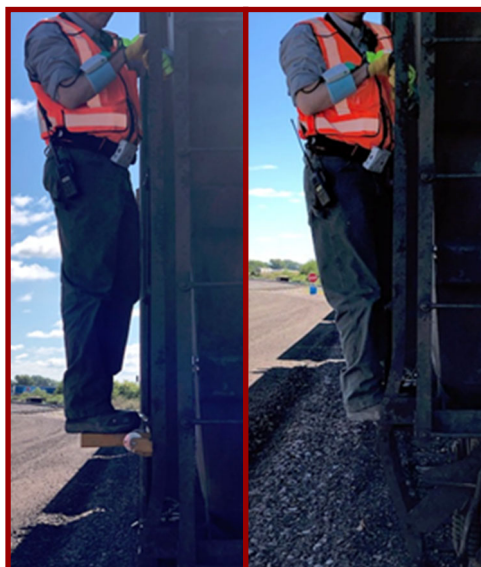
Riding on a ladder with (left) and without (right) a riding platform.
