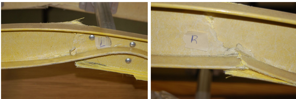
Figure 3. Failure of the extension ladder's rails
