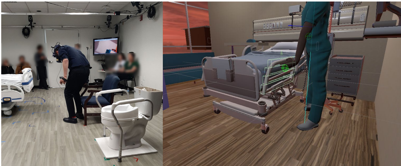
Figure 1. (Left) Image of mixed reality trials using virtual display and physical objects for creating immersive experience within a hospital room modeled after existing room architecture. (Right) A virtual environment with collision boxes highlighted on the hospital bed side rail for collecting proximity data during immersion.
