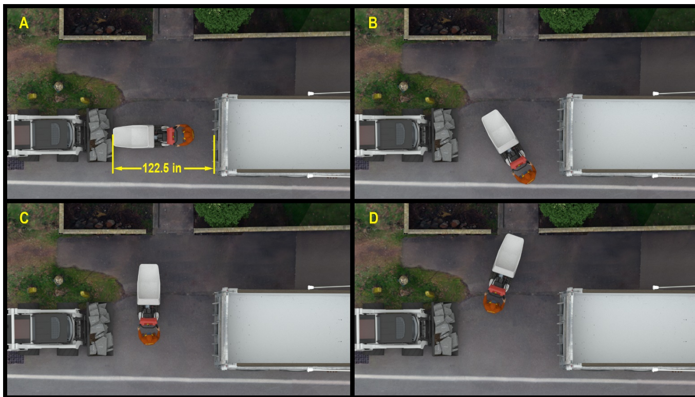
Figure 5. Alternate Safe Work Procedure Using Two-Point Turn to Prevent Rear Contact with Dump Truck
