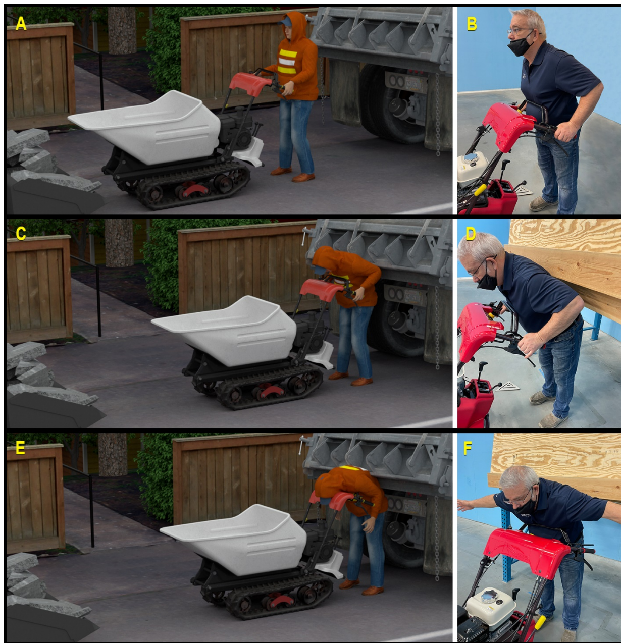
Figure 4. 3D Computer Model Analysis (Left) and Human Surrogate Studies (Right) of Accident
