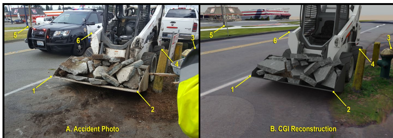
Figure 2. Camera Match Points for Convergence of Accident Site Geometry
