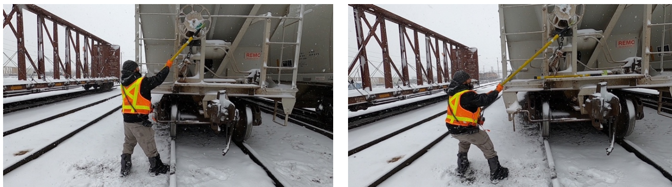
Figure 2. A short brake stick results in poor biomechanics and fouling the red zone (left). A long brake stick nurtures proper biomechanics and staying clear of the red zone (right).
