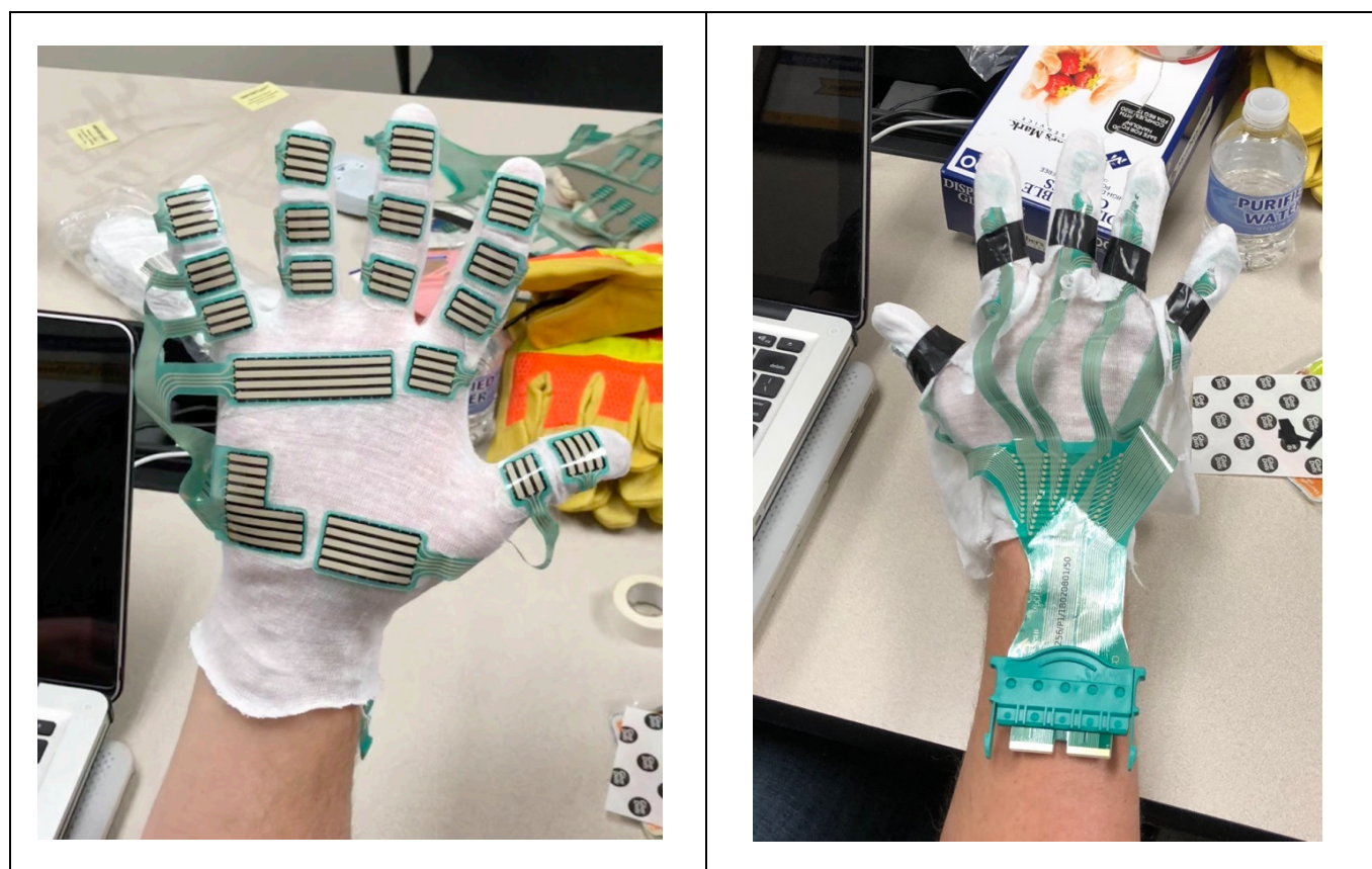
Figure 1. Tekscan palm-side hand force sensors assembled to thin cotton glove on the left; the rest of the “circuit board” on the right
