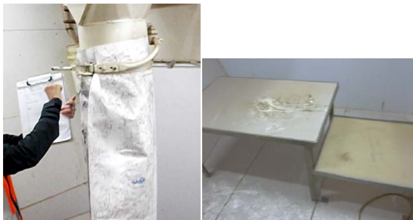
Figure 2. Bag Filling Station. Table below filler (left) 22" H; scale on lower surface (right) is ~20"H, not pictured
