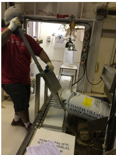
Figure 12. Push-lever bar to transition the fish meal bag from upright to side-lying in the correct orientation to feed into the bag squeezer.
