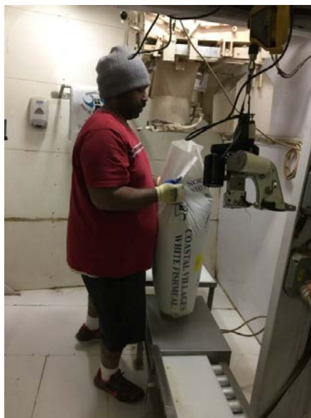
Figure 8. Sewer suspended on tool balancer. No ramp between bag filler table and scale surface; bag is dragged.
