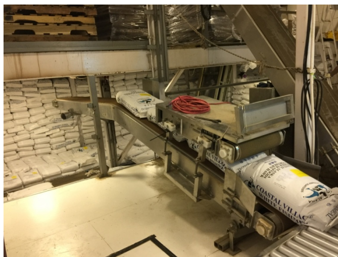
Figure 11. Automated bag squeezer on existing powered conveyor to the lower storage level.
