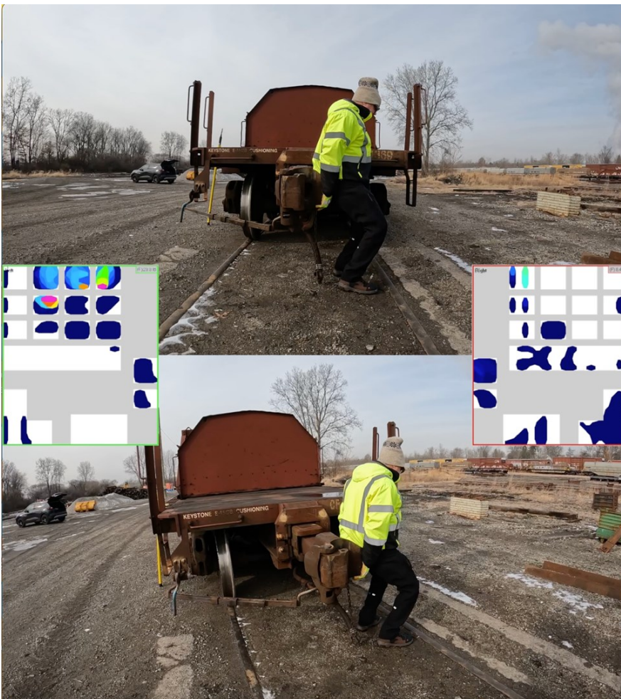
Drawbar adjustment using the "back into" method; pressure mapping for each hand and associated hand forces (28.8 lbs.—right hand; 8.4 lbs.—left hand).
